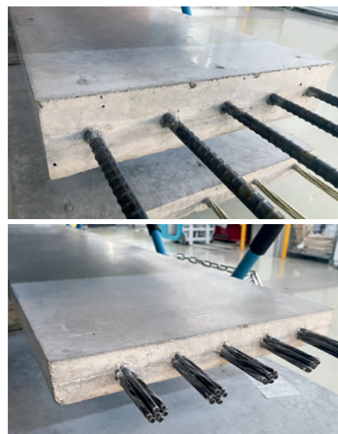
Figure 1 FRP-rebar reduces the amount of concrete used.
