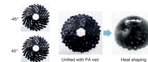
Figure 2 Example of a dome preform using resin A towpreg
