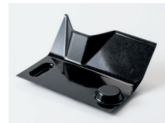
Figure 2 Test moulding of 3D shapes (rCF-mat / Arkema Elium®)
