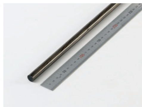
Figure 2 Prototype CF/PP rod (Φ 13 mm, Vf 60%) produced by high-speed pultrusion molding
